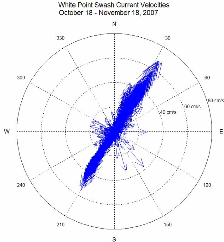
**Figure 8. Compass plot of the current velocities from the ADCP approximately 50 cm above the creek bed throughout the entire deployment. The creek orientation was approximately 33 degrees east of north. Dominant current direction was in the along-channel direction, and strongest currents were observed during the flooding tide.**
