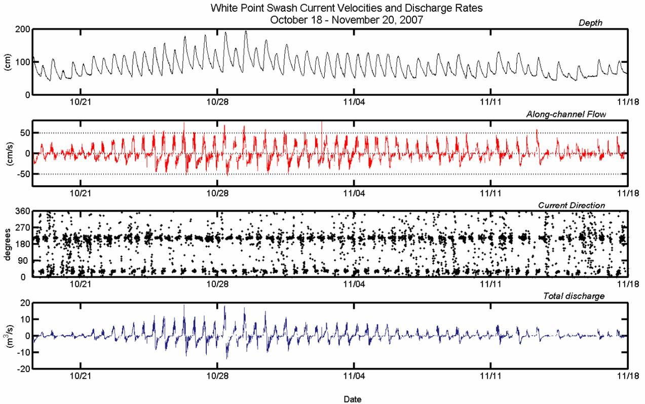
**Figure 7. White Point Swash water level, along-channel currents, current direction, and discharge rates across the channel for the entire deployment period.**
