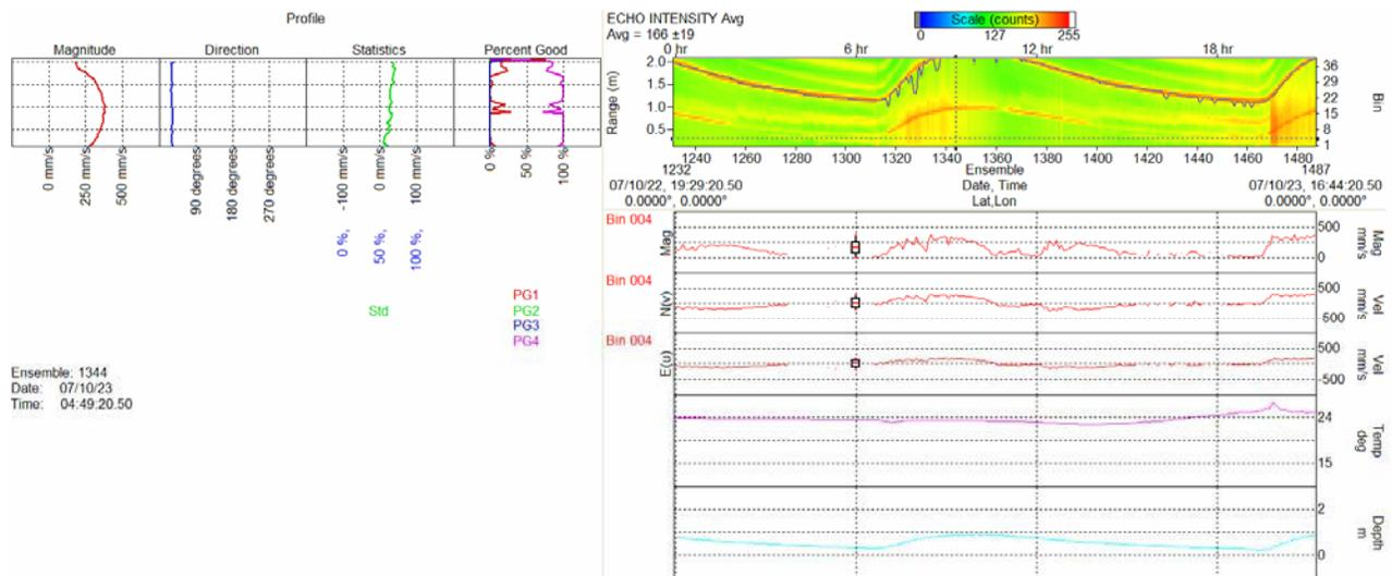
**Figure 6. Snapshot of raw ADCP echo intensity data in the viewing software WinADCP. The first high return in the contour plot is the actual surface of the water column.**
