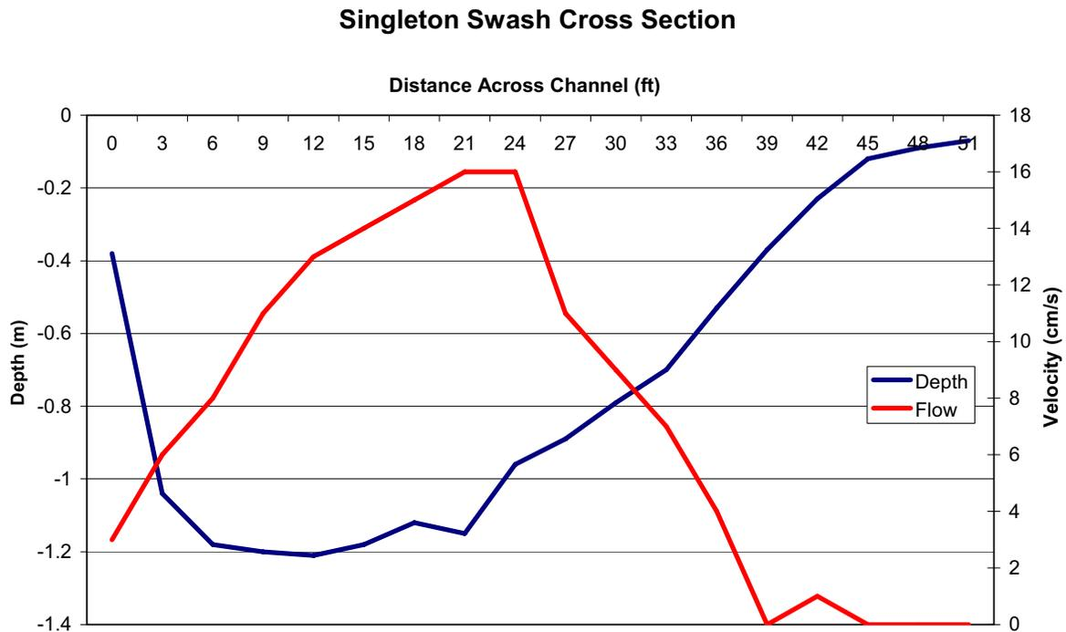
Figure 2. Current magnitude and depth across the creek channel where the ADCP was deployed. The zero distance across the channel is the north side of the channel.
