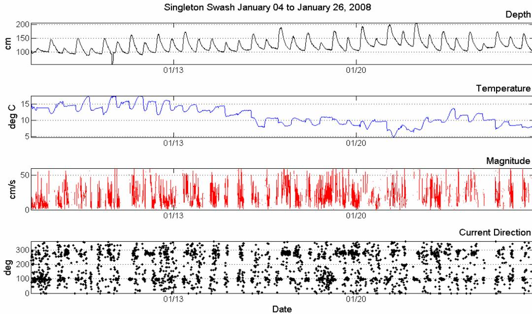
**Figure 6. Singleton swash water level, measured temperature, current magnitude, and current direction in the channel for the entire deployment period.**
