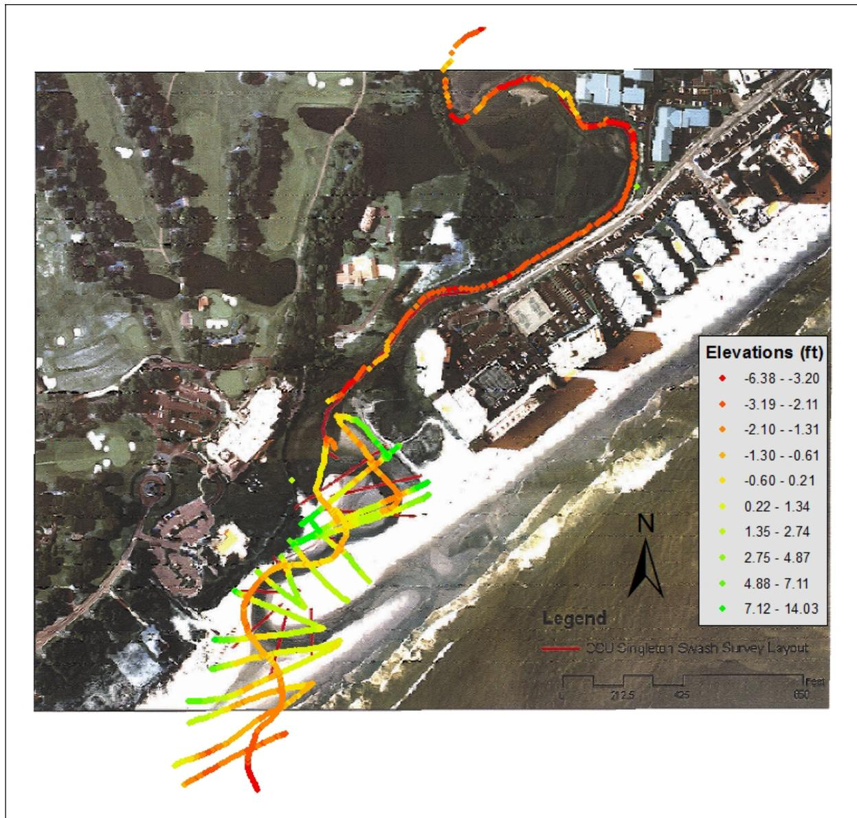
Figure 1. GIS interpretation of the survey data overlaid onto an aerial photo of the study site. Shallow depths appear in yellow, while the deeper channel can be seen as the darker red.
