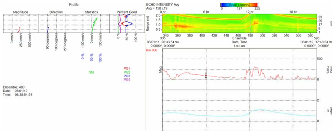
**Figure 5. Snapshot of raw ADCP echo intensity data in the viewing software WinADCP. The first high return in the contour plot is the actual surface of the water column.**
