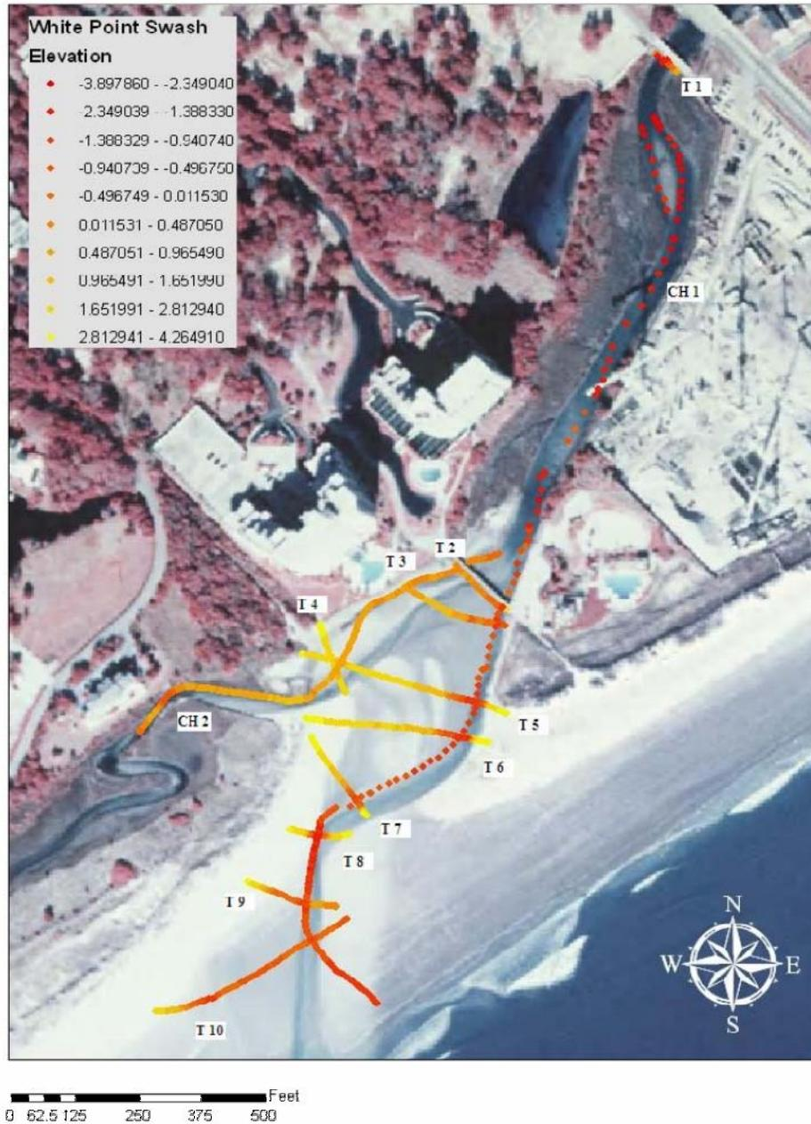
Figure 2. GIS interpretation of the survey data overlaid onto an aerial photo of the study site. Shallow depths appear in yellow, while the deeper channel can be seen as the darker red.
