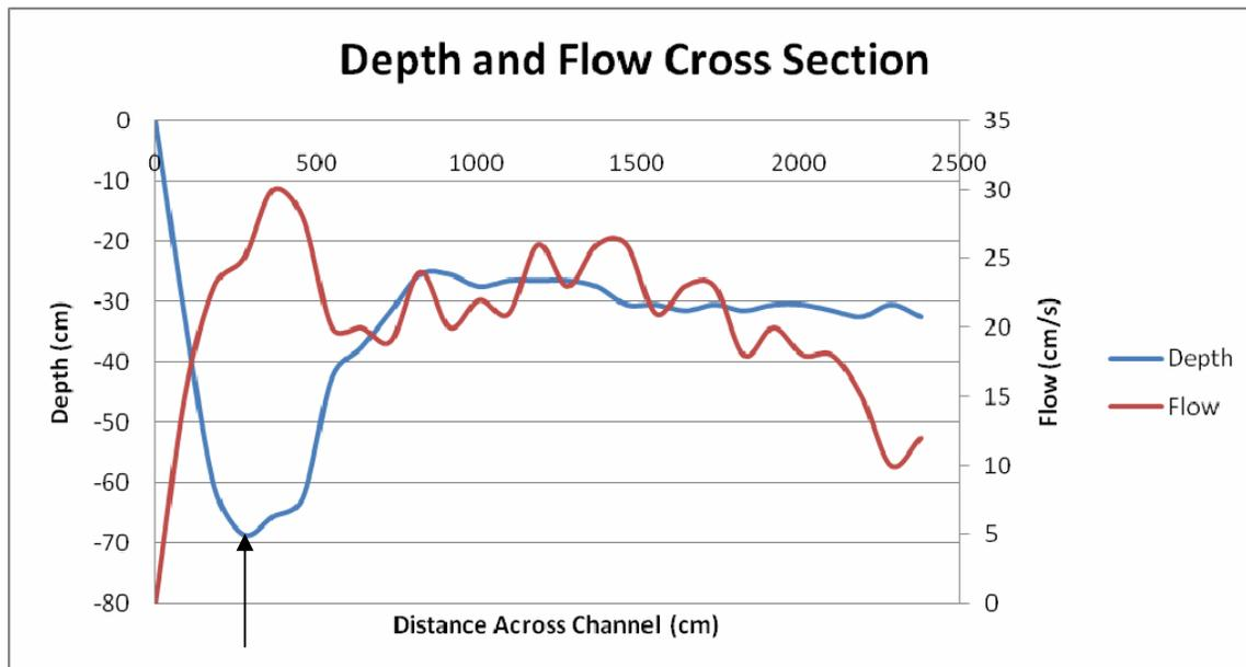
Figure 3. Current magnitude and depth across the creek channel where the ADCP was deployed. The arrow indicates the location of the ADCP within the cross section.
