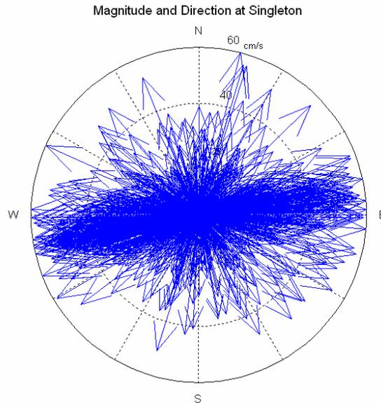
**Figure 7. Compass plot of the current velocities from the ADCP approximately 50 cm above the creek bed throughout the entire deployment. The creek orientation was approximately east – west and the dominant current direction was in the along-channel direction.**
