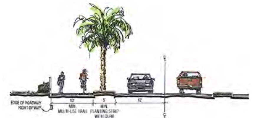
Typical cross-section of the East Coast Greenway in unincorporated Horry County. Source: East Coast Greenway Master Plan for Horry and Georgetown Counties (pictured below)
