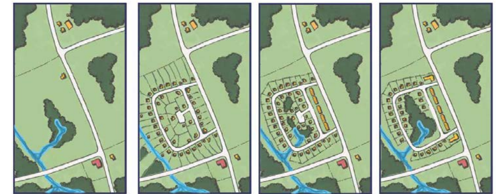
Example conceptual designs showing pre-residential development, traditional residential development design and two versions of Conservation Subdivision Design
