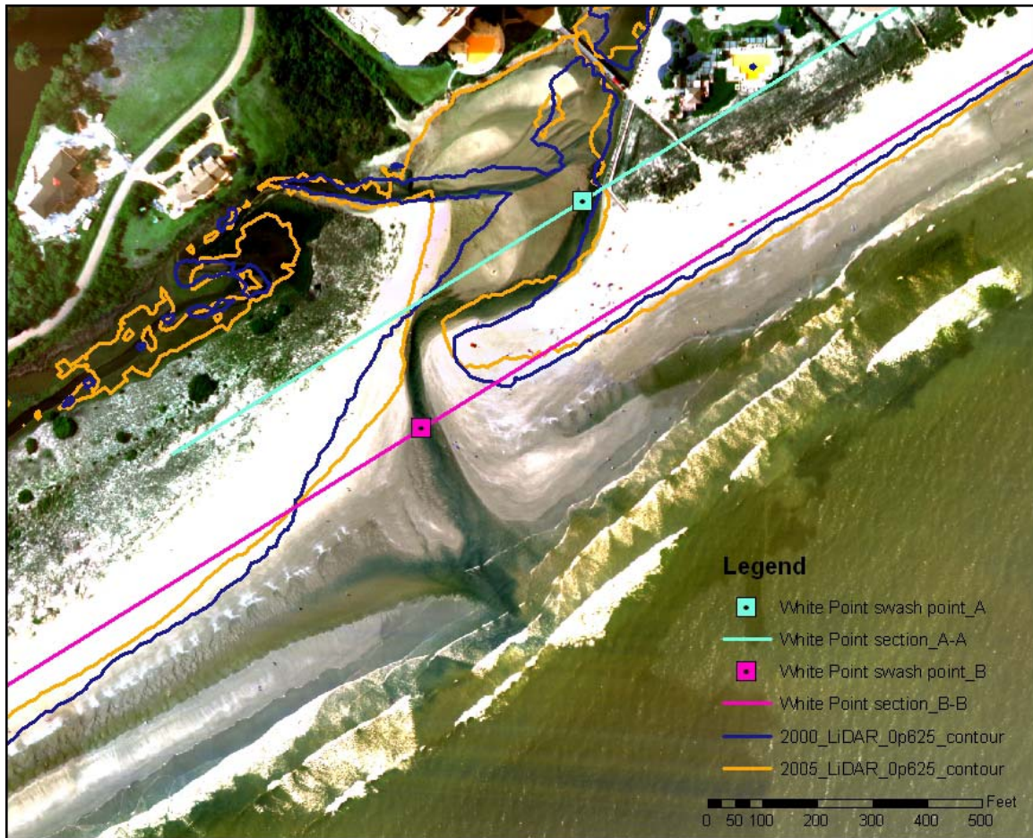
Figure 6-14: +0.625 meter LIDAR elevation contour comparison for 2000 and 2005 at White Point Swash.
